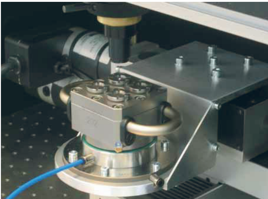
Chuck height: only 23 mm!
