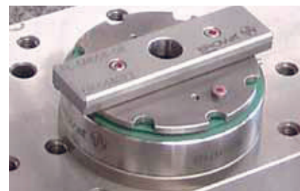
All axes, X, Y, Z and the center are checked with the same alignment plate.
