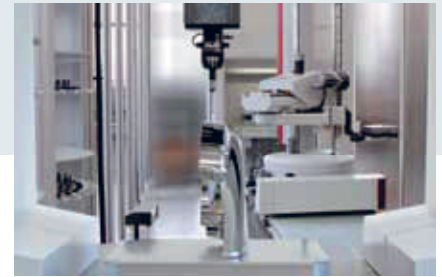
03 | The handling facility serves the measuring station with manufactured products for interim and final checks.
