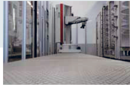
02 | The stable linear rail is extended to the required length in segments.
