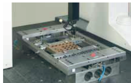
Presetting made easy. While the WEDM center is in operation, the next job is being preset quickly and accurately on the EROWA PreSet station.
