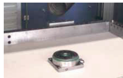
The chucks can be fitted to the machine table directly or with adapter plates.
