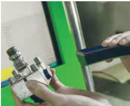
On the set-up and measuring stations, hand-held reading devices are used. (The EWIS™ Rapid equipment is available as an option).
